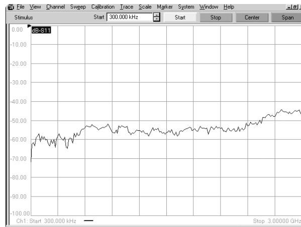
Figure 11. Measurement of load standard after calibration
